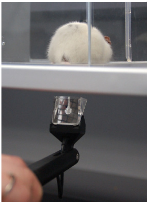
Fig. 1: "touch stimulator" transducer, including prism Grid mesh not included (optional)
